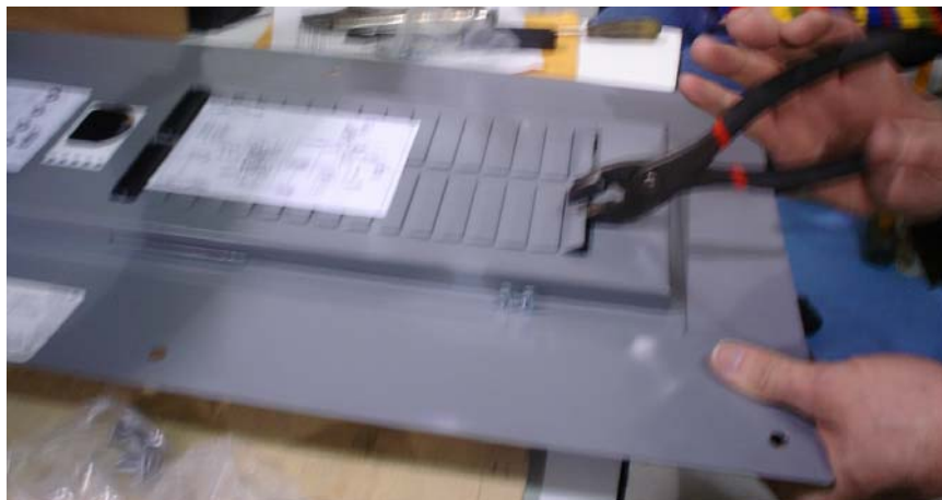
Pliers used to remove knockout from back of door mechanism
