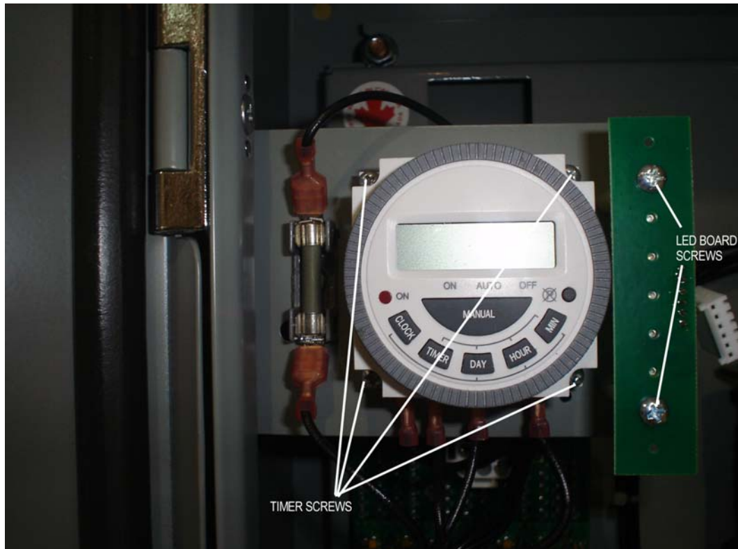
Figure 8. TIMER AND LED BOARD SCREWS
