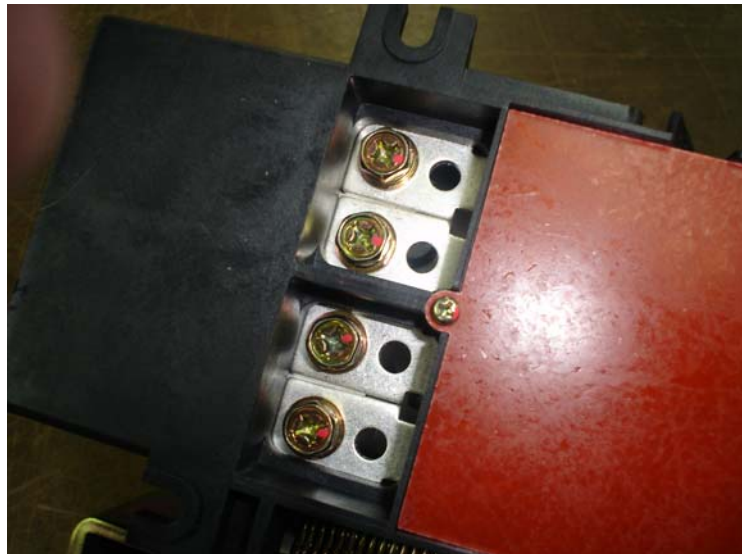
Figure 7. UNDERSIDE OF SWITCH SHOWING THE LOAD LUG ADAPTOR PLATE SCREWS
